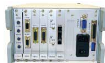
Model 1560 has 6 slots for modules
