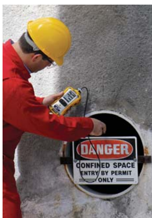
Confined space testing with the MultiRAE Lite
