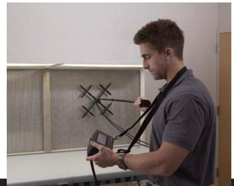
Plug and play thermoanemometer probes enables use in multiple applications.
