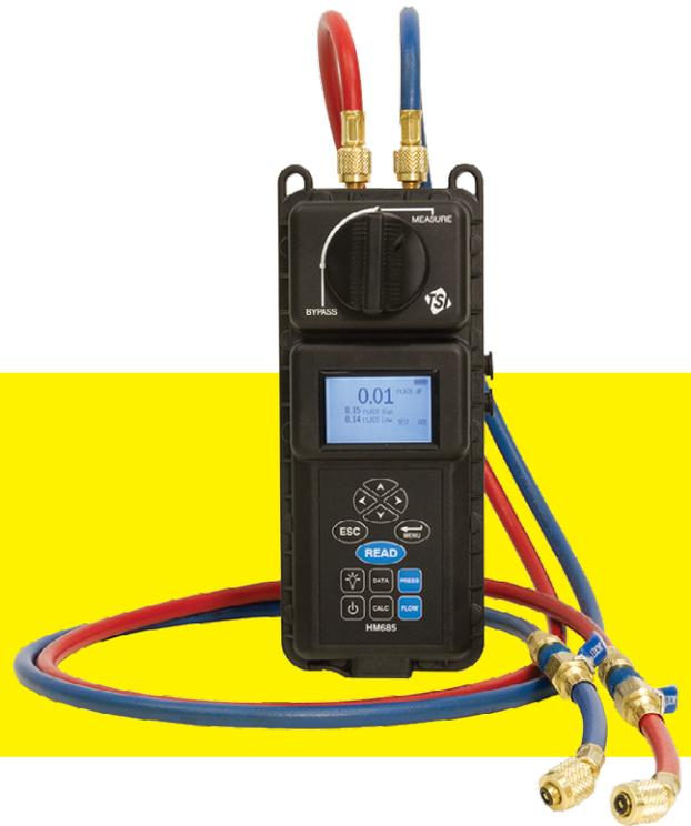
The HM675 and HM685 Hydronic Manometers are used to balance hydronic heating and cooling systems, check pump performance and to set balancing valves. They can measure and display differential, high side and low side pressure simultaneously, without having to change hose connections or instrument valve settings. Each model features a backlit display and operates on four alkaline or NiMH rechargeable batteries.
